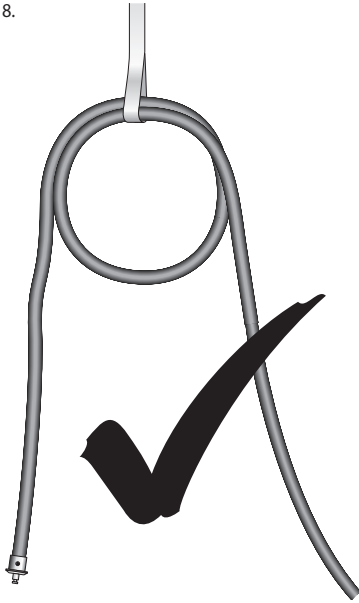
Correct method of hoisting HVSC Plus
