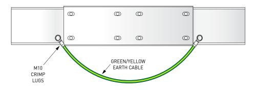
LPI offers an extensive range of cable earth bonds and flexible tinned copper braids for the electrical earthing of cable ladder, conveyors, handrails, metal cladding, water pipes, fences and gates.
