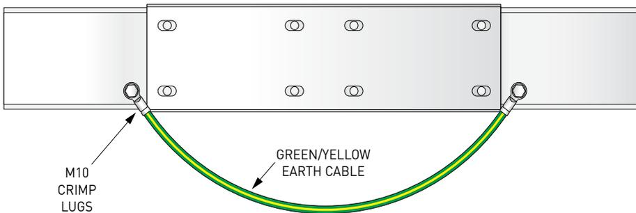
LPI offers an extensive range of cable earth bonds and flexible tinned copper braids for the electrical earthing of cable ladder, conveyors, handrails, metal cladding, water pipes, fences and gates.
